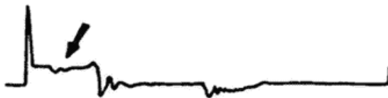
Mixture ration is too lean or cylinder pressure is too low
