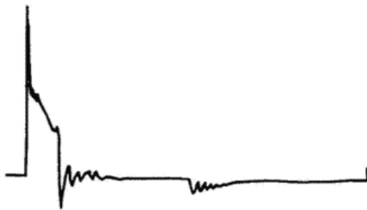
Secondary circuit resistance is too large
