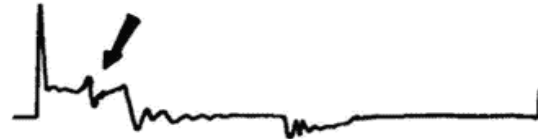
Distributor cover or distributor lead is matched un-tightly
