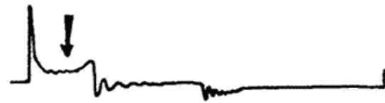
Mixture ratio is too rich or spark plug leak electricity
