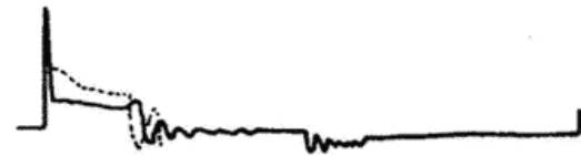
Injector of electronic fuel injection poor work
