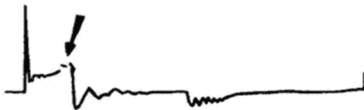
Spark plug overheated or valve guide leakage
